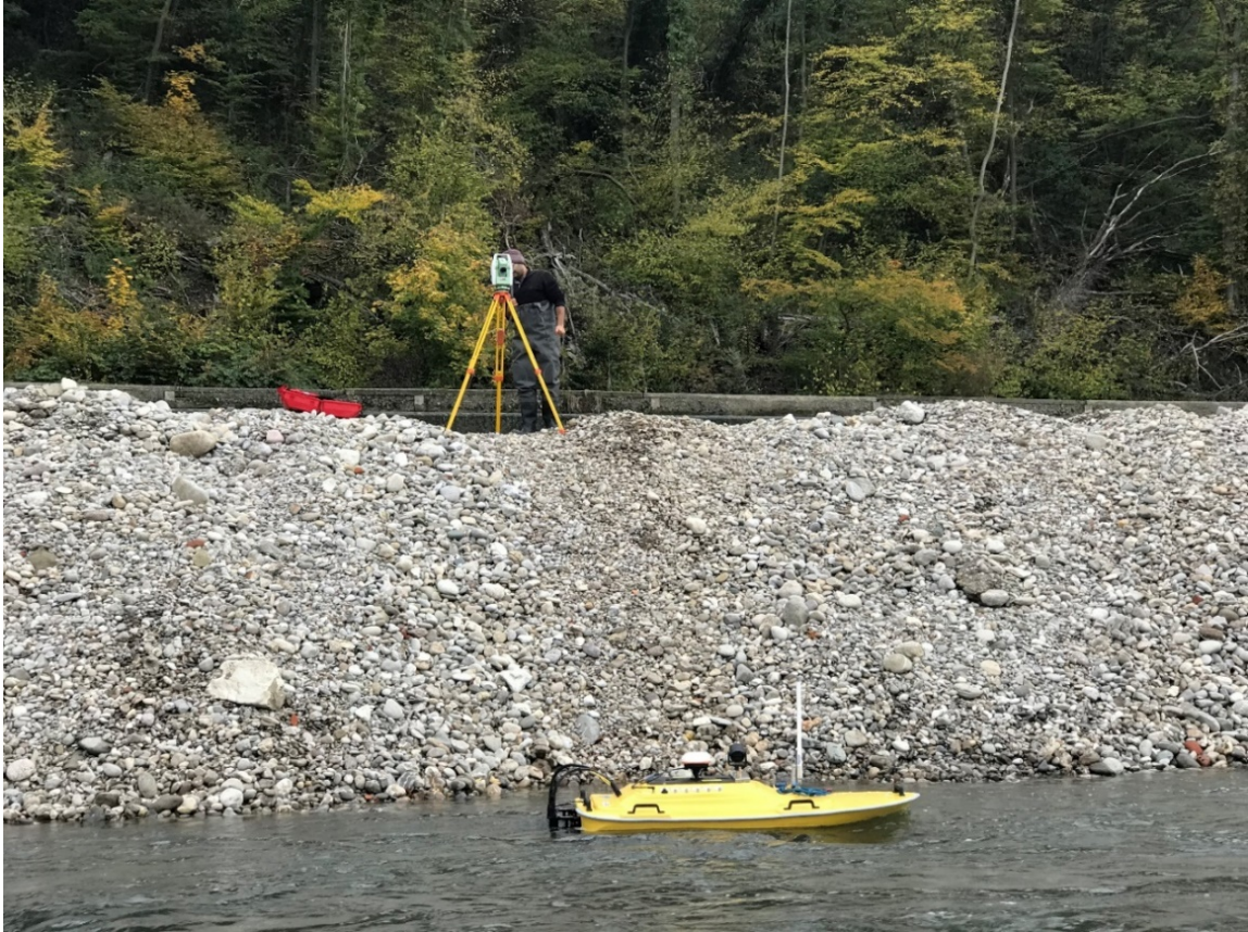
Figure 36: Water surface elevation measurements using a total station and a target on the boat
