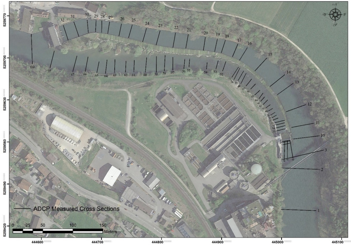
Figure 35: Velocity and bathymetry measurement locations at HPP Schiffmühle in October 2018.
