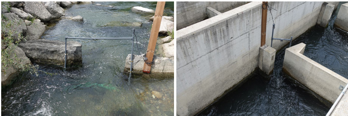
Figure 39: PIT-Tag antennas (left picture in the nature-like fish pass, right picture in the vertical-slot pass).
