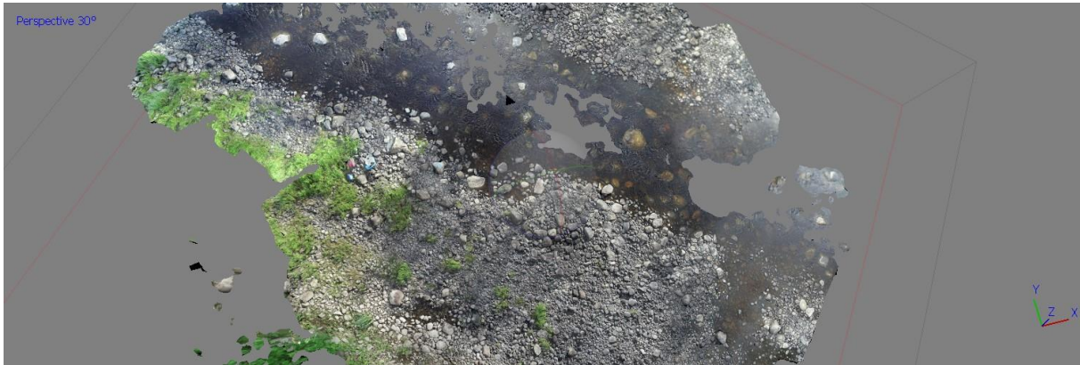
Figure 10: SfM measurements in the residual flow reach to evaluate the roughness of the gravel areas
