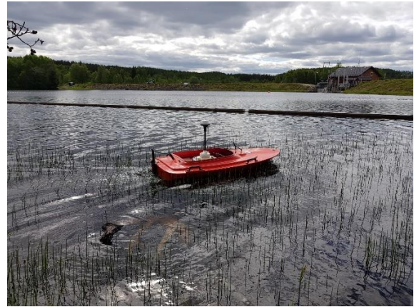
Figure 8 : The Sontek M9, one mounted on a kayak (left) and an autonomous boat (right)
