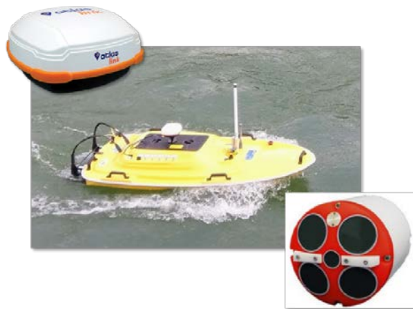
Figure 7: Teledyne Marine Q-boat of VAW equipped with ADCP probe and GPS antenna
