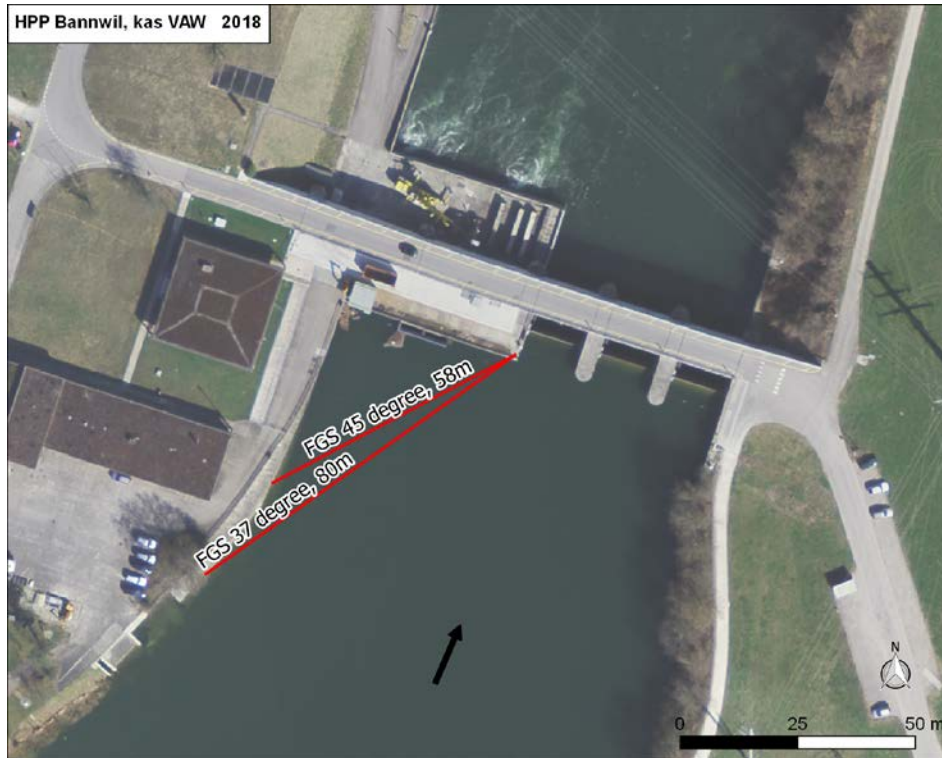
Figure 21: Potential positions of fish guidance structures upstream of the HPP Bannwil (background image: © 2018 swisstopo (JD 100041))
