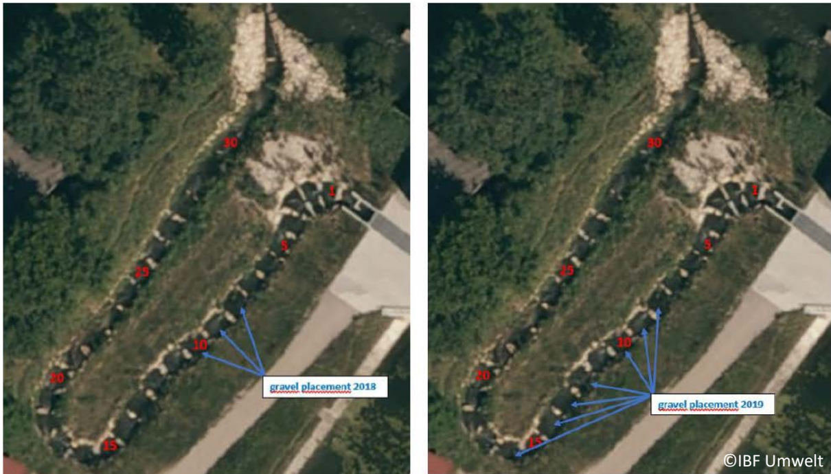
Figure 12: Location of gravel input at the fishway Wattenweiler in 2018 (left) and 2019 (right)
