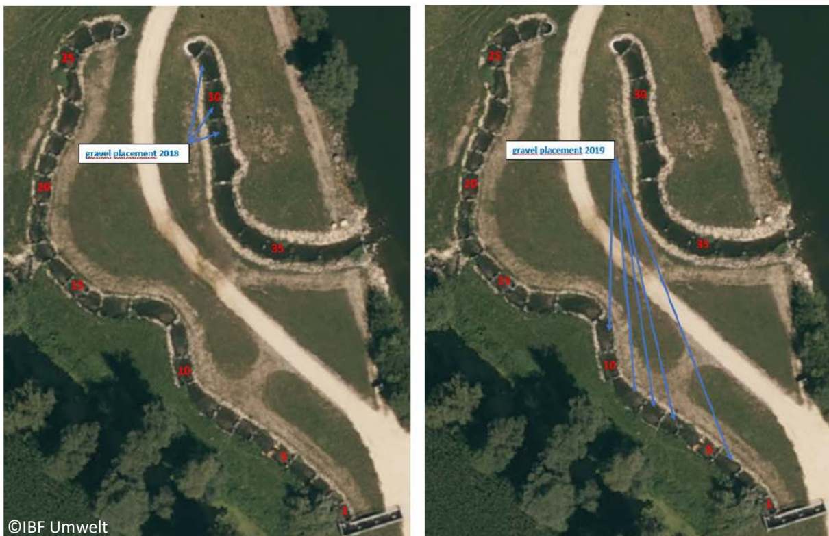
Figure 13: Location of gravel input at the fishway Ellzee in 2018 (left) and 2019 (right)
