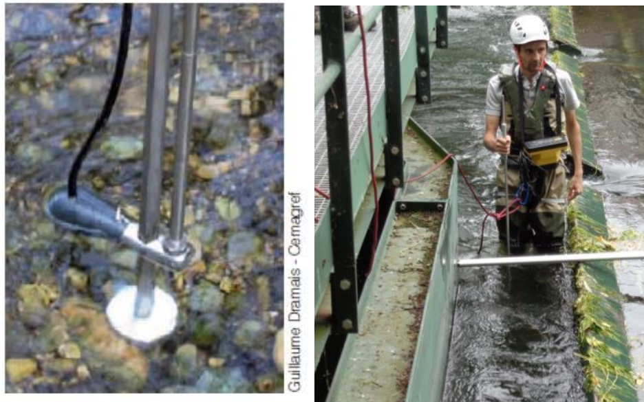
Figure 46: Example of an electro-magnetic flow meter and an operator in position in the downstream migration duct
