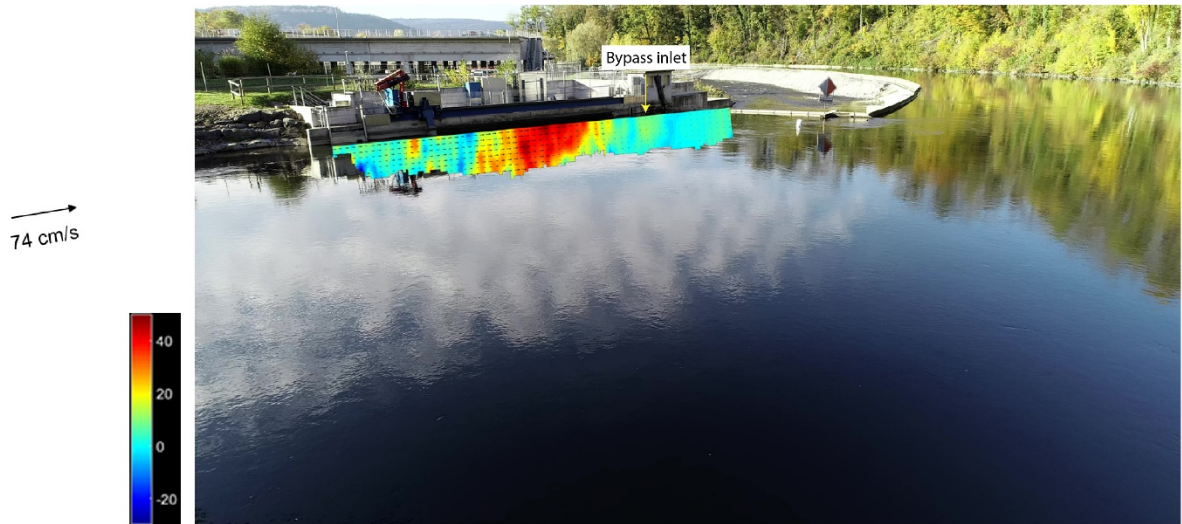
Figure 37: Velocity distribution along the HBR-BS in October 2018.
