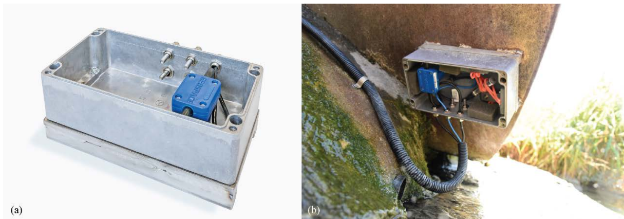
Figure 10: The bedload monitoring setup with (a) the housing and the geophone and (b) the housing mounted to the vortex tube and all sensors installed.
