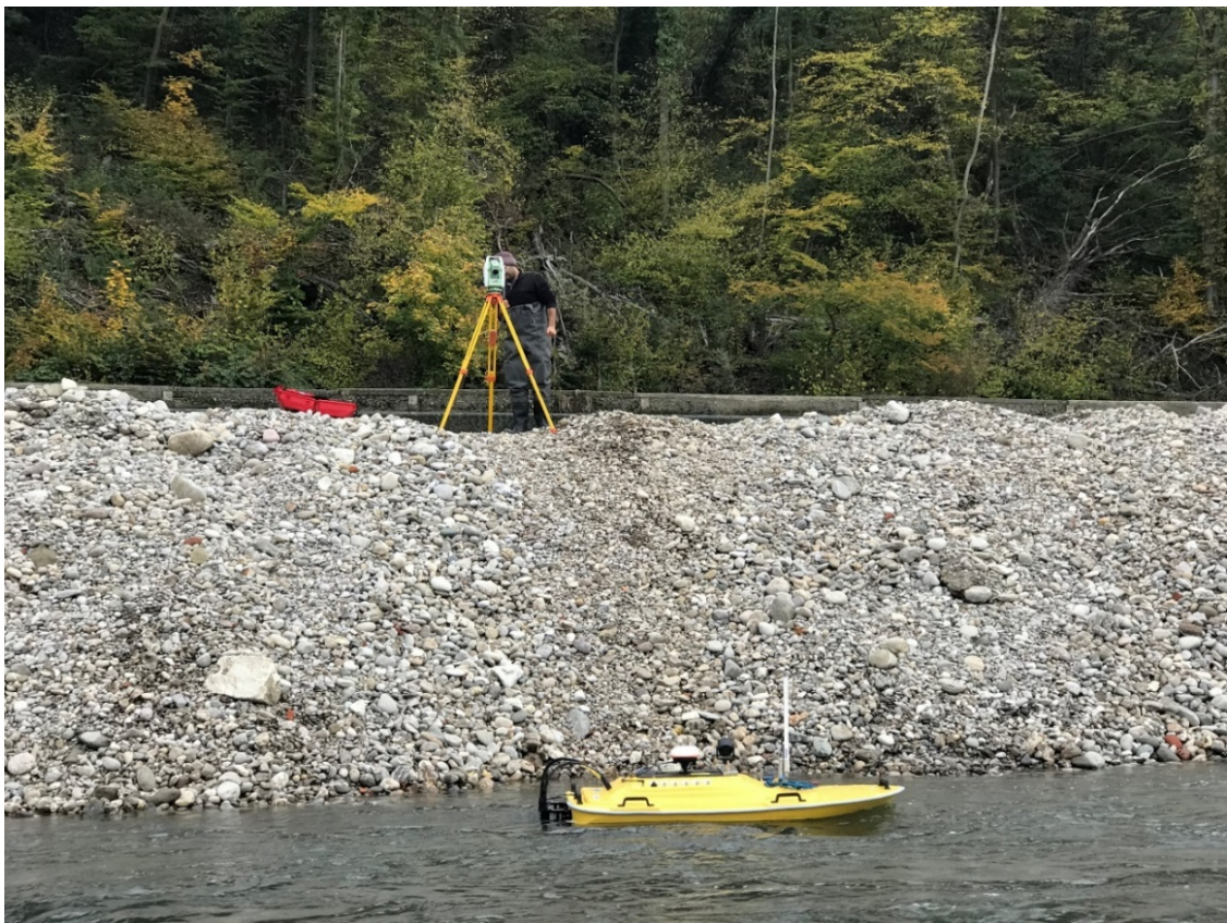
Figure 25: Water surface elevation measurements using a total station and a target on the boat
