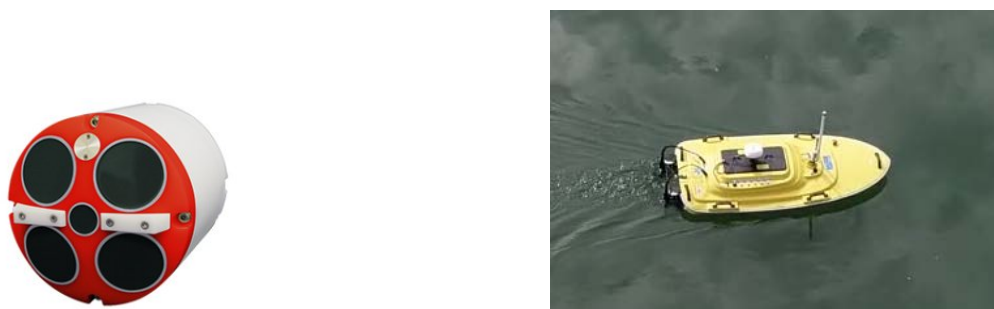
Figure 21: ADCP and Q-boat
