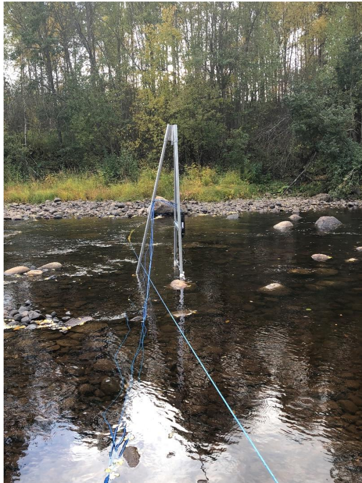
Figure 9 : ADV measurements in the bypassed reach
