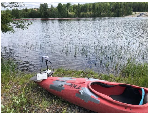
Figure 8 : The Sontek M9, one mounted on a kayak (left) and an autonomous boat (right)
