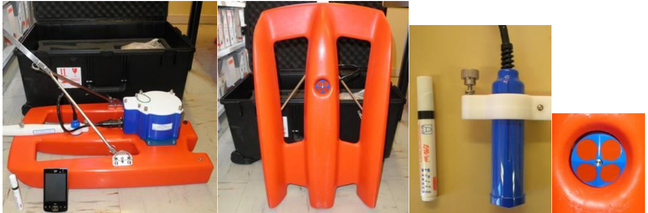
Figure 39: Pictures of the ADCP StreamPro assembled on its trimaran and the probe with a closer view of the 4 sensors
