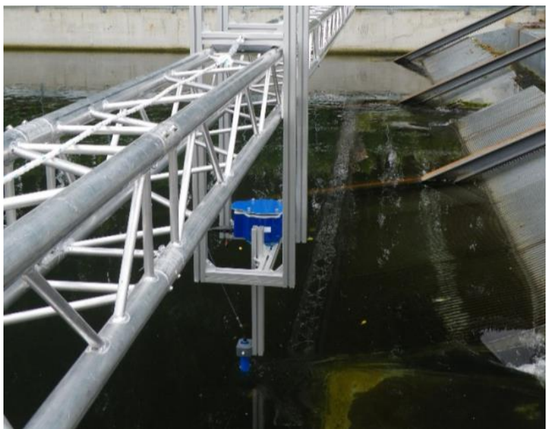
Figure 40 : Support and movement carts system allowing the deployment of the ADCP
