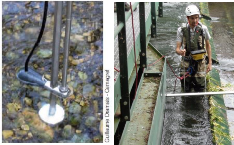
Figure 44: Example of an electro-magnetic flow meter and an operator in position in the downstream migration duct
