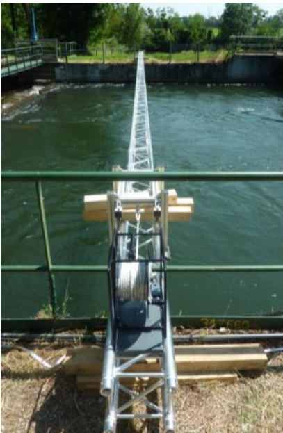
Figure 40 : Support and movement carts system allowing the deployment of the ADCP
