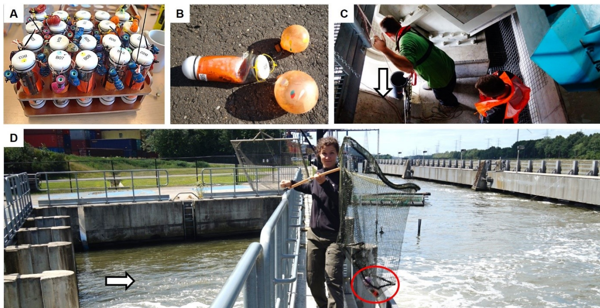
Figure 12: BDS deployment at Ham from 20-22.06.2018. A) Sensors outfitted with balloon tags ready for deployment. B) Sensor destroyed by crush event. C) Deployment of BDS into the Archimedes screw. D) Recovery downstream via balloon tags in a hand net.
