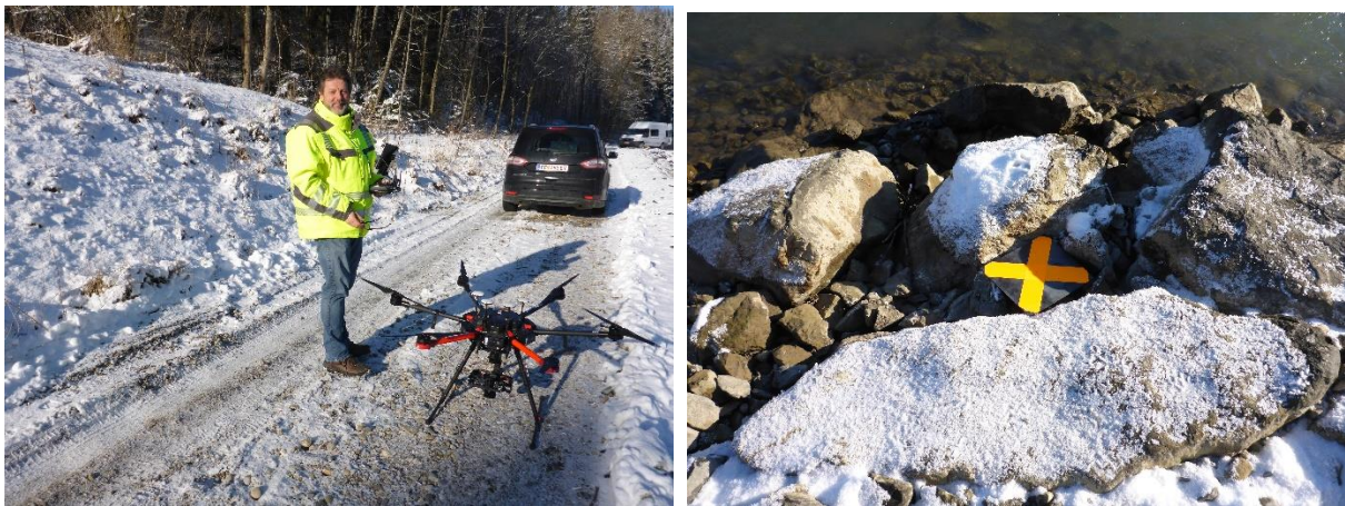
Figure 6: Drone used for the aerial survey (left), Ground control point (GCP, right)
