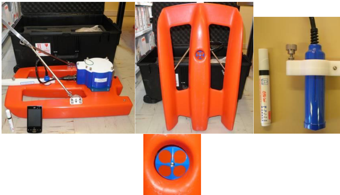
Figure 15: Pictures of the ADCP StreamPro assembled on its trimaran and the probe with a closer view of the 4 sensors
