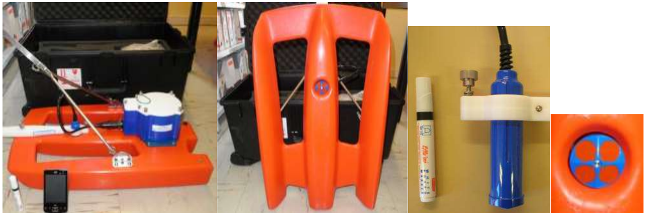
Figure 41: Pictures of the ADCP StreamPro assembled on its trimaran and the probe with a closer view of the 4 sensors
