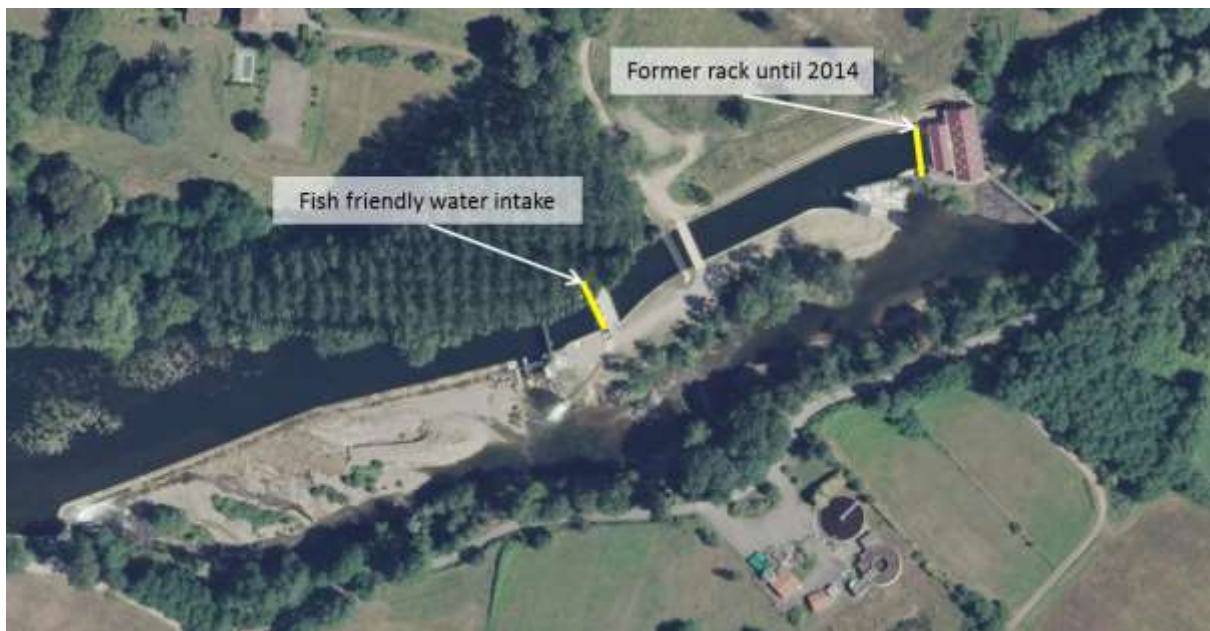
Figure 10: Positioning of downstream migration devices
