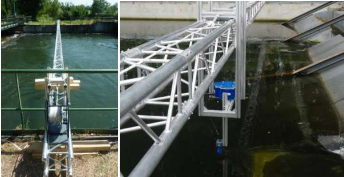
Figure 42 : Support and movement carts system allowing the deployment of the ADCP
